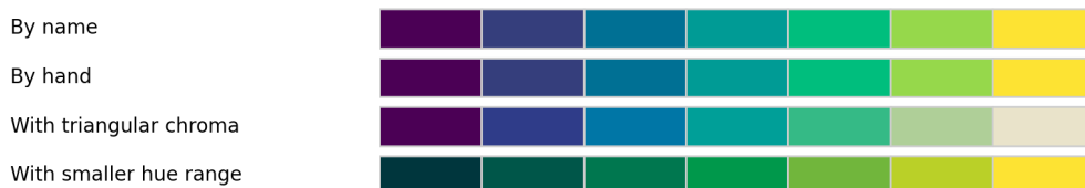
Figure 1: Swatches of four HCL-based sequential palettes: pal1 is the predefined HCL-based viridis palette, pal2 is identical to pal2 but created “by hand” and pal3 and pal4 are modified versions with a triangular chroma paths and reduced hue range, respectively.
