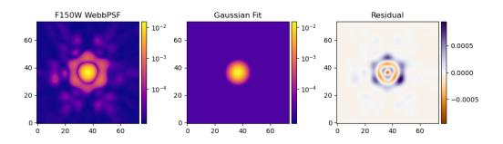
**Figure 2:** The plot on the left shows an idealized forward model of the NIRCam F150W PSF made using WebbPSF. The middle shows a Gaussian approximation to the PSF. The right shows the residual between the WebbPSF model and the Gaussian approximation.
